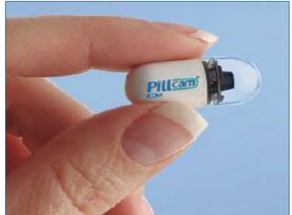
The PillCam® SB 2 video capsule.
